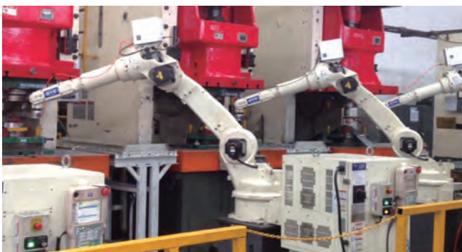
Transfer between presses
